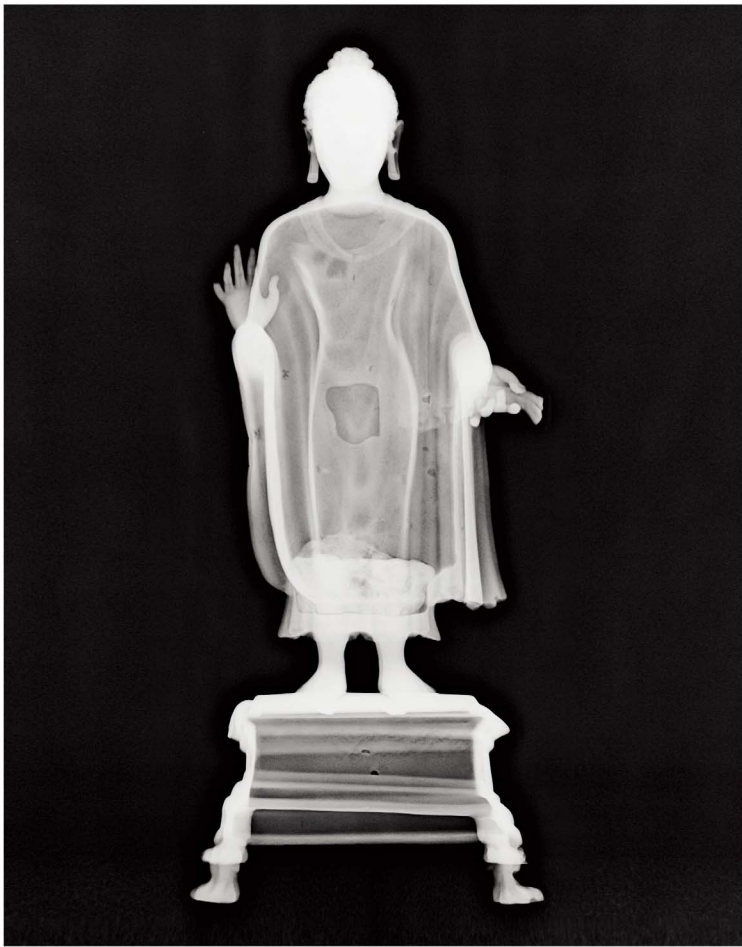
22 X-ray radiograph, frontal view, Nelson-Atkins Museum of Art (44-13) (21). © Nelson-Atkins Museum of Art. An opening in the back wall is visible, in addition to a large cast-in repair at the bottom of the robe. There are no internal gates and there appears to be no armature inside this figure
