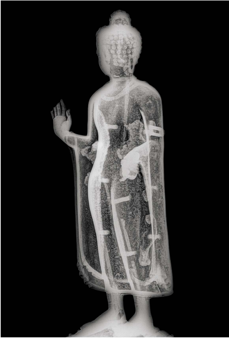
17 Computed radiograph, three-quarter view, digitally enhanced, Cleveland Museum of Art (1968.40) (7). © Cleveland Museum of Art. The internal gates are visible as radiopaque, i.e. white bands. Extant lengths of the armature are visible in the head, chest and legs, with less easily discernable, more corroded, sections in the torso
