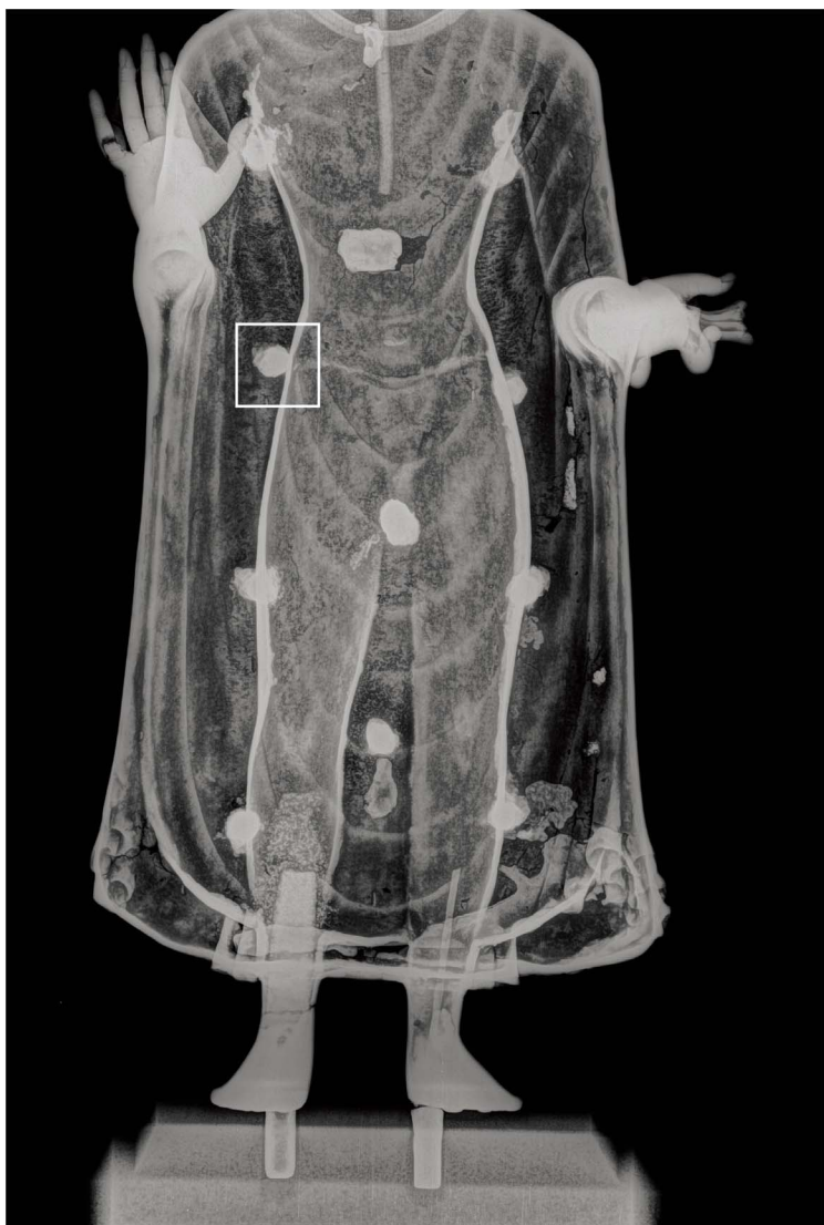
15a Computed radiograph, frontal view, digitally enhanced, The Metropolitan Museum of Art (69.222) (2, 4). Photograph by The Department of Objects Conservation. Image © The Metropolitan Museum of Art. Ten internal gates are visible in areas of the robe as radiopaque, i.e. white, circles, four cast-in repairs are visible and the figure's right foot is a modern restoration. Four cast-in lead repairs to front of the proper left side of the robe are seen as a string of radiopaque round and elongated patches
