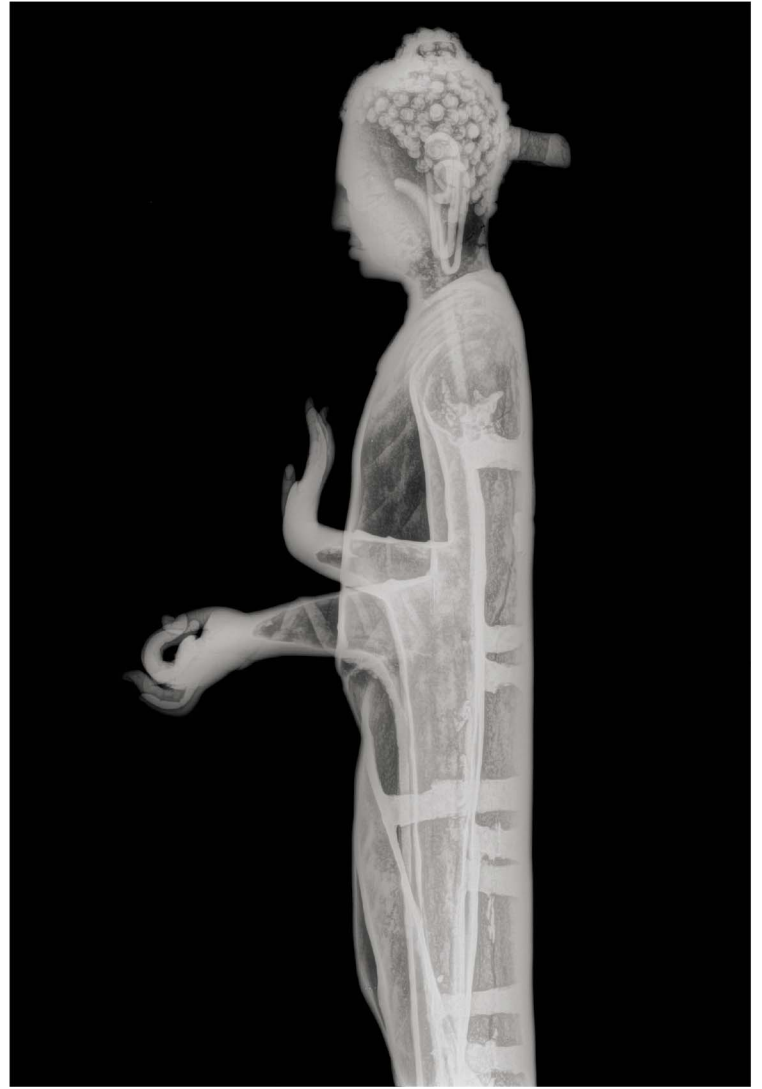
18 Computed radiograph, profile view, digitally enhanced, The Metropolitan Museum of Art (69.222) (3). Photograph by The Department of Objects Conservation. Image © The Metropolitan Museum of Art. The internal gates are visible as radiopaque, i.e. white, bands. An extant section of the iron armature is visible in the head and chest
