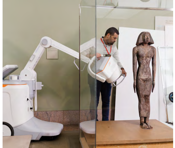
Ahmed Tarek using a portable X-ray machine on the statue of Mitry's wife (26.2.3) to determine how best to remove it from its mount
